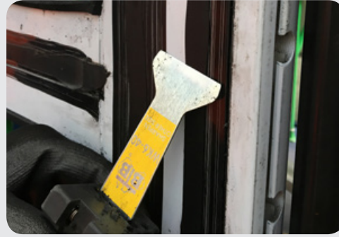
BTB Trim Blades to Remove Excess Sealant on Frame/Body Panel
